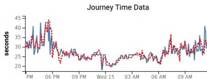
Figure 3: An example of aggregated journey time data for a section of the A59 plotted in blue, versus our fitted model with 30-minute predicted journey time plotted in red
